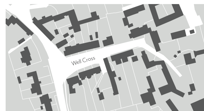
Edith Weston Historic Core figure ground plan showing semi-detached, terraced and farmyard buildings, with a much more direct relationship to the street, mostly set at 90 degrees but sometimes at odd angles
